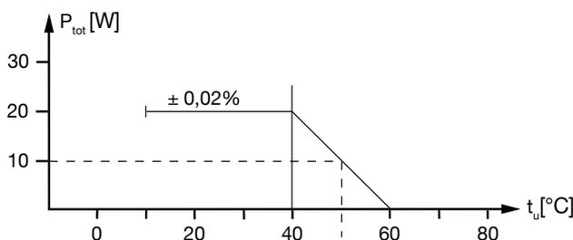
The max. load capacity with different ambient temperature as a function of the warm-up error can be taken from the load reduction curve. **Example:** Ambient temperature: max. 50°C; accepted ΔR by temperature influence: max. 0.02 %; max. permissible load: 10 W.
