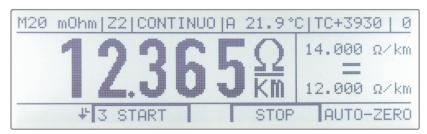
Measurement at a cable drum with measurement value indication  $\Omega/m$ ,  $\Omega/km$  as well as  $\Omega/km$  and  $\Omega/km$ . Entry of the cable length 0.01 meter up to 9999 meter is possible.
