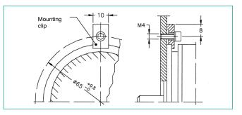
1 set of mounting angles with screws (3 are part of delivery) for model 8820-5350 and 8820-5350-V501 Model 8820-Z002
