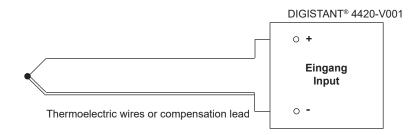
The reference junction is located inside the device (internal). It is simulated electronically by a built-in Pt100 sensor.
