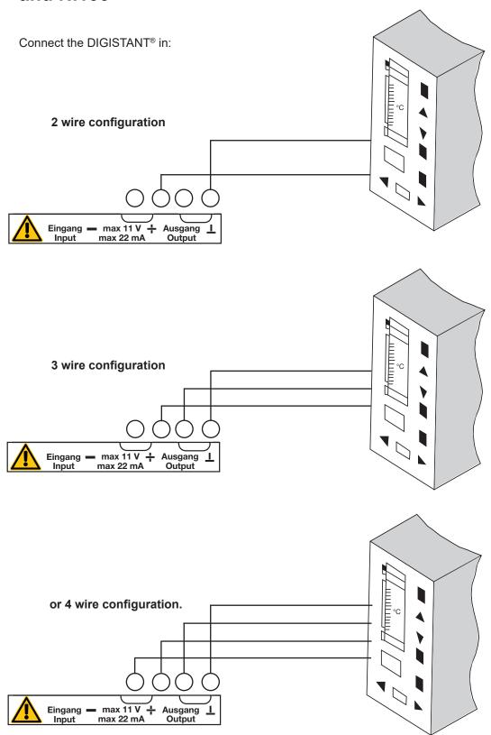
Switch on the device and connect it as shown above.
