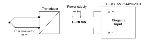
Switch on the device and connect it as shown above.
